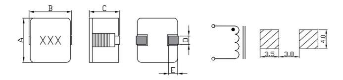
$A = 10.20 \pm 0.50 \text{m/m} \; ; \; B = 10.50 \pm 0.50 \text{m/m} \; ; \; C = 4.20 \text{m/m} \; MAX; \; D = 2.00 \pm 0.50 \text{m/m}; \; E = 2.00$
