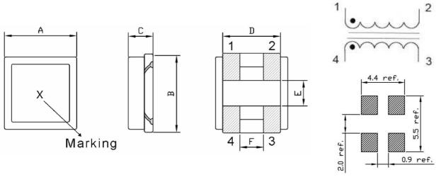
A=4.80 $\pm$ 0.30 m/m ; B=5.00 $\pm$ 0.30 m/m ; C=2.50 m/m Max (do not include solder); D=3.50 m/m Ref. E=2.20 m/m Ref. ; F=1.10 m/m Ref.
